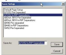
...give your **Page Setup** a name which reflects the press size and if necessary the **Separations Style** so it will be easy to select later.
