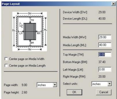
• Check that the **Media Width**, **Media Length** and **Margins** are correct for your plate. (The calibration target is rather small, but you should check to ensure the margins will put it inside your printing area).
