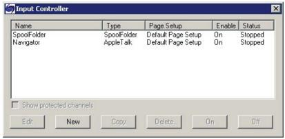
The Input Controller dialogue box shows the input sources currently available. Each input source can be turned on or off individually using the buttons— the state is displayed in the **Status** column.
