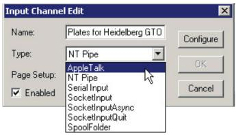
The AppleTalk Input Plugin is one of the simplest to set up, and there is nothing that needs to be configured for this plugin, so you can now click **OK** and the plugin is ready to use.
