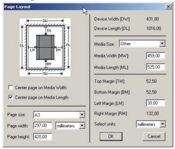
..edit the existing Media Width and Media Length settings to reflect the plate size of your new press page setup.
