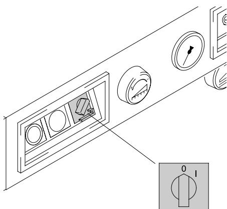
Replacement of blade and cutting stick may be performed only when the main switch is switched off!
