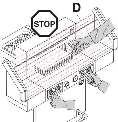
It is forbidden to operate the machine if the operating and safety instructions have not been understood. Please check the safety devices are functioning and complete before use.
